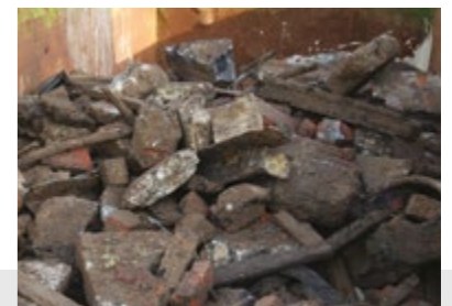
Deponieaushub Rollend > 200 mm
